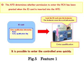
The APD has a slot into which the ID card is inserted, and communication is enabled by inserting the ID card into the APD.
