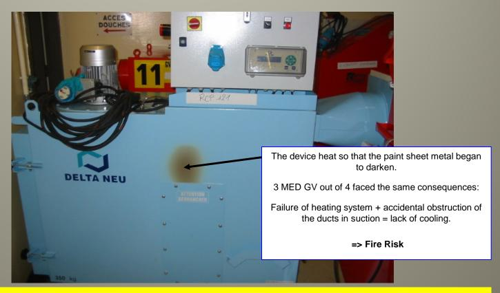
**REX :** Two evacuations of the reactor building during outages in 2011 and 2012: smoke detection ... Problem of MEDGV (*PVU used on Steam Generator Pipe Head during Eddy currents*)
