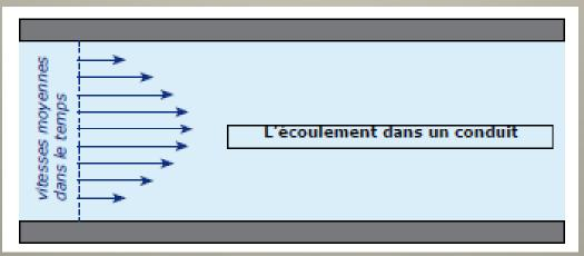
The average speed in the duct section is 5.89 m/s, in the center a maximum value is 18 m/s (duct diameter : 300 mm and air flow 3000 m<sup>3</sup>/h).
