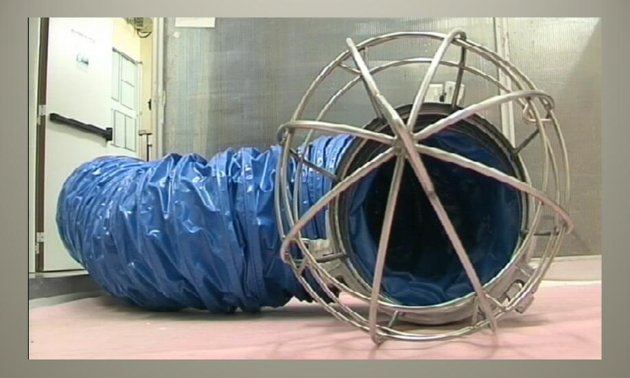
The sphere cage can be adapted to different duct diameters. The ZAG couplings will then be used for DN 300, 200, 170 or 150.
