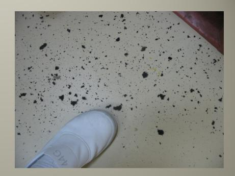
Incandescent particles (insulation material) were projected from the outlet. • The material temperature (post filter and lodine trap) increased by convection through the metal casing (separating the heating system of discharging casing). The temperature was high enough to carbonize and reach the point of ignition.
