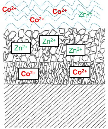
Increase of Co-58 and Co-60 in the primary water coolant is expected when the addition of DZO (depleted zinc oxide) is started!
