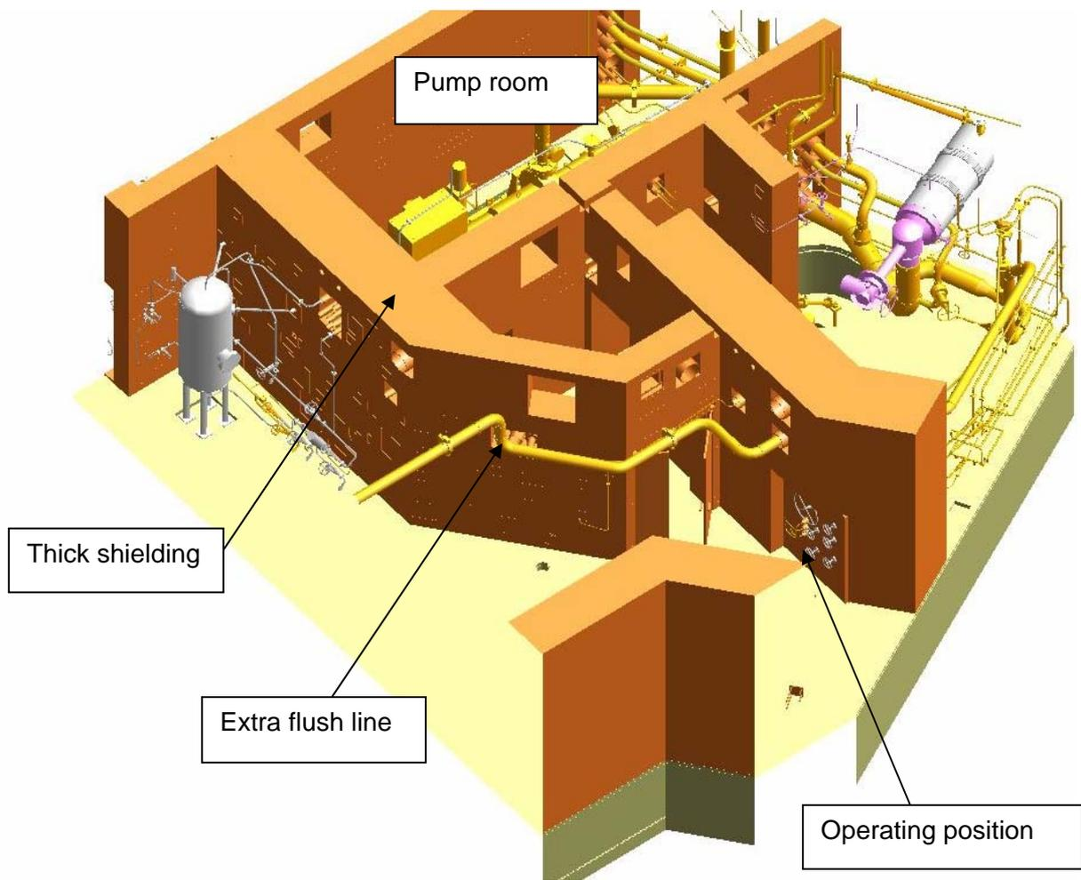
Figure 5. Design features in the Safeguards Building for post-accident management
