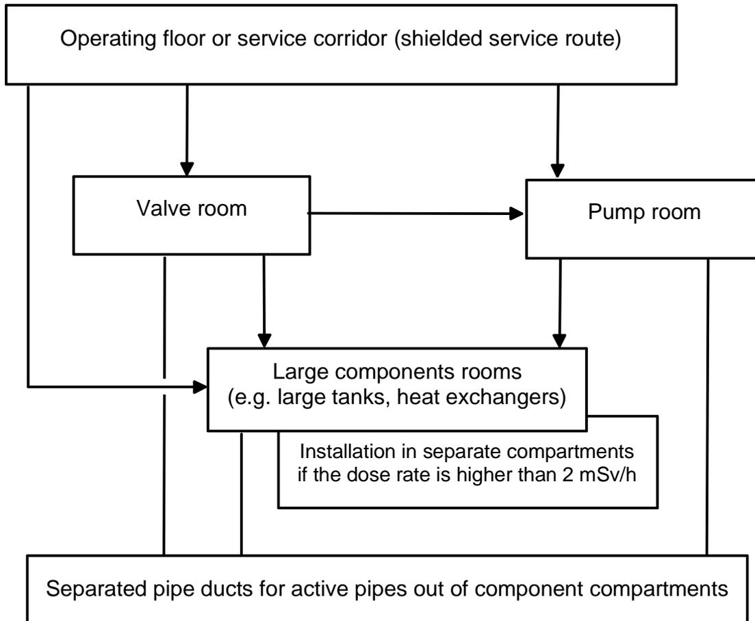
Figure 3: Principle scheme of compartment access
