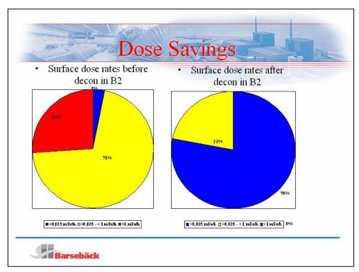
Figure 10: Changes in dose rates before and after the decontamination in Unit 2
