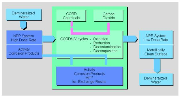
Figure 2: Principle of the HP/CORD UV Concept
