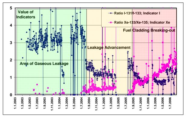
Fig. 4. Fuel cladding leakage indicators at Temelin NPP Unit 2 between 2003 and 2006
