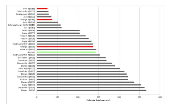
Figure 6 - (Inter)national comparison of RVCH replacement projects. In red, the Belgian replacement projects and in green, the average value of all reported replacement projects [2][3][4].
