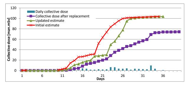
Figure 4 - Comparison between collective dose after replacement and estimated collective dose for the Tihange 3 project.
