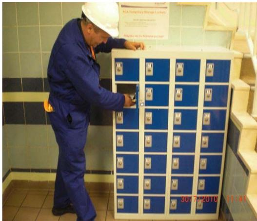
Lockers on route to the Radiation Controlled Area (RCA) to support the Pocket Restriction Policy ie only take the items you require for the job into a RCA.
