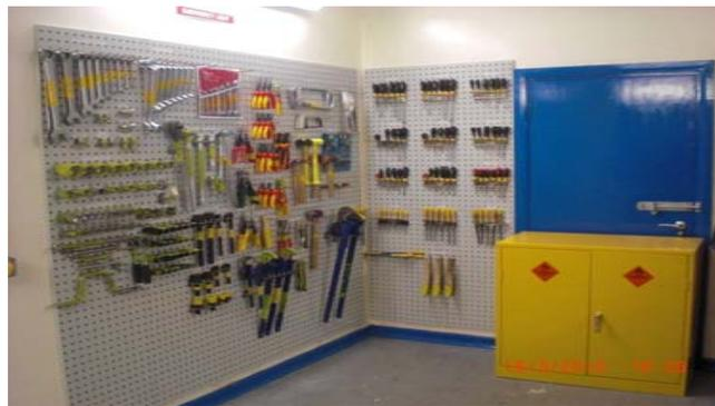
Radiation Controlled Area tool stores: Not having to remove tools from the RCA reduces the risk of inadvertently spreading contamination beyond the RCA boundary and improves all-round productivity.
