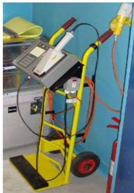
Standard portable instrument for personnel to monitor themselves at temporary Contamination Controlled Area (C2) barriers.
