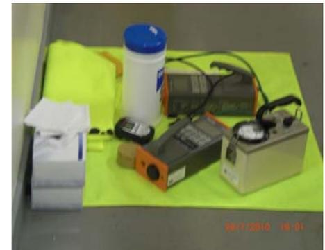
Laundryable contamination control mats: To provide a clean working surface in a Contamination Controlled (C2) Area.
