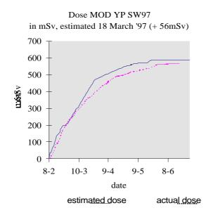
Figure 1: The dose planned and the dose realised as a function of the time allocated to the operations relating to the modification of the primary safety valves.
