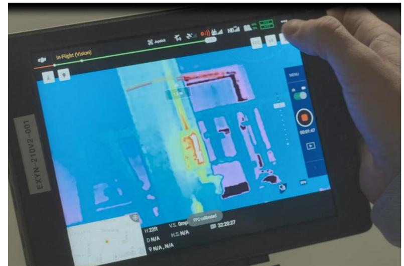
Thermal Camera on Drone Detects Heat Blanket Remotely
