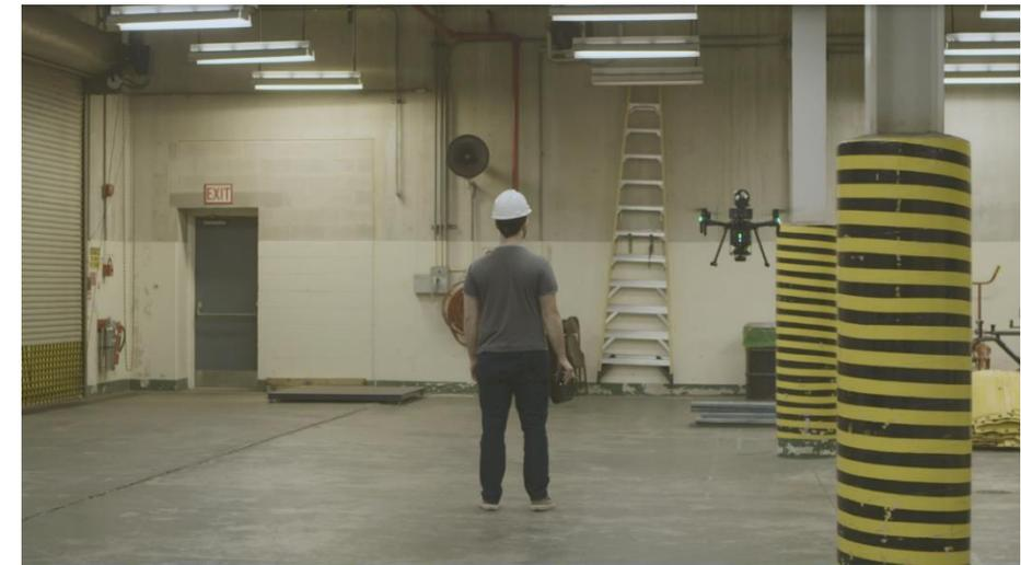
Drone Detects and Autonomously Rerouted Around Obstacle
