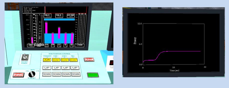
To determine the real time reactor response to operator actions, Point reactor kinetics with simplified thermal feedback model is implemented
