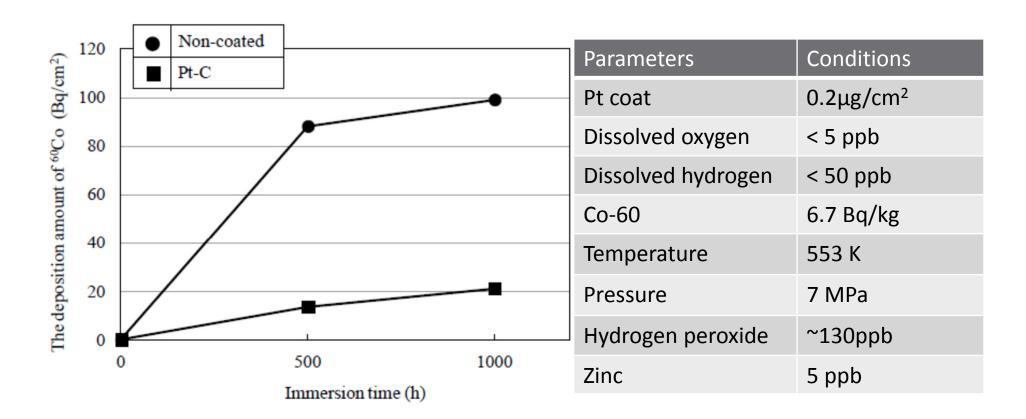
The immersion time dependency of 60Co deposition amount under BWR condition.
