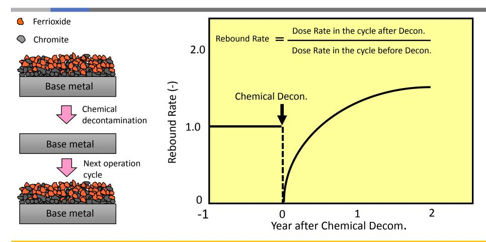
After the chemical decontamination, the surface of the piping is restored to the original condition as time elapses.
