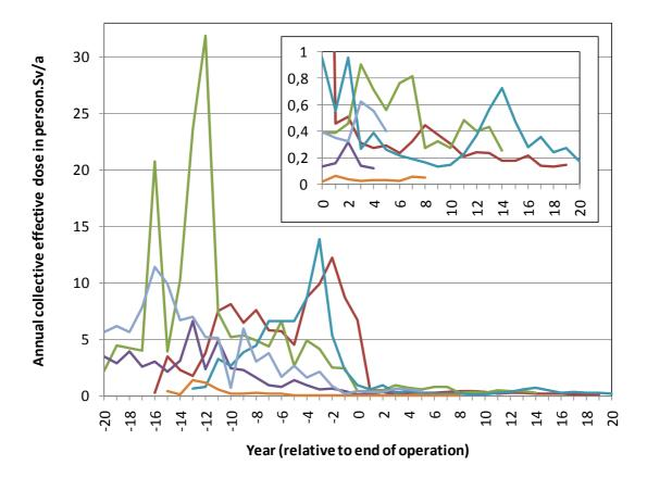
**Fig. 7:** The annual collective effective dose of several German NPPS, plotted relative to the end of the operation (insert: magnification of the decommissioning phase)
