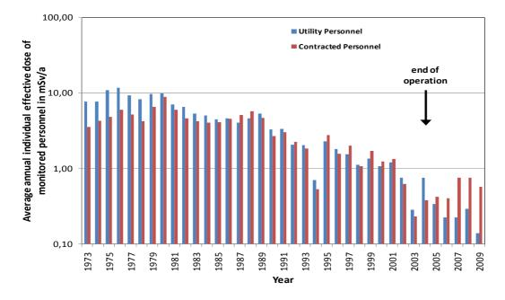
**Fig 6:** The average annual individual effective dose in mSv/a during operation and decommissioning of an arbitrarily chosen German NPP
