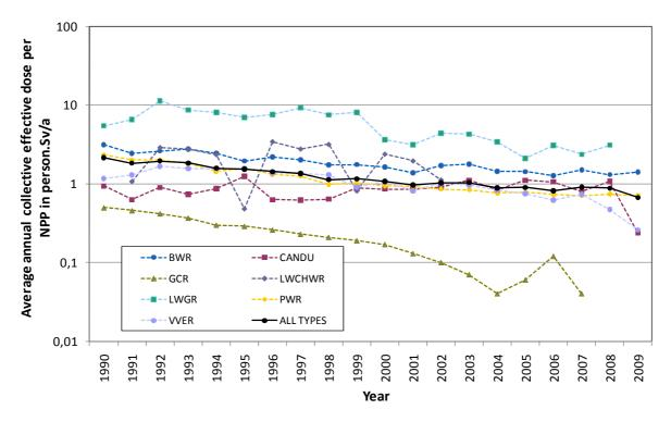
**Fig 1:** The average annual collective effective dose per (operational) NPP of a reactor type in person.Sv/a during the last 2 decades
