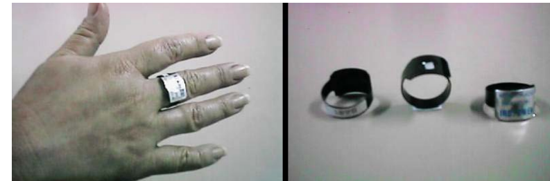
IRD TLD extremity individual monitor (ring)
