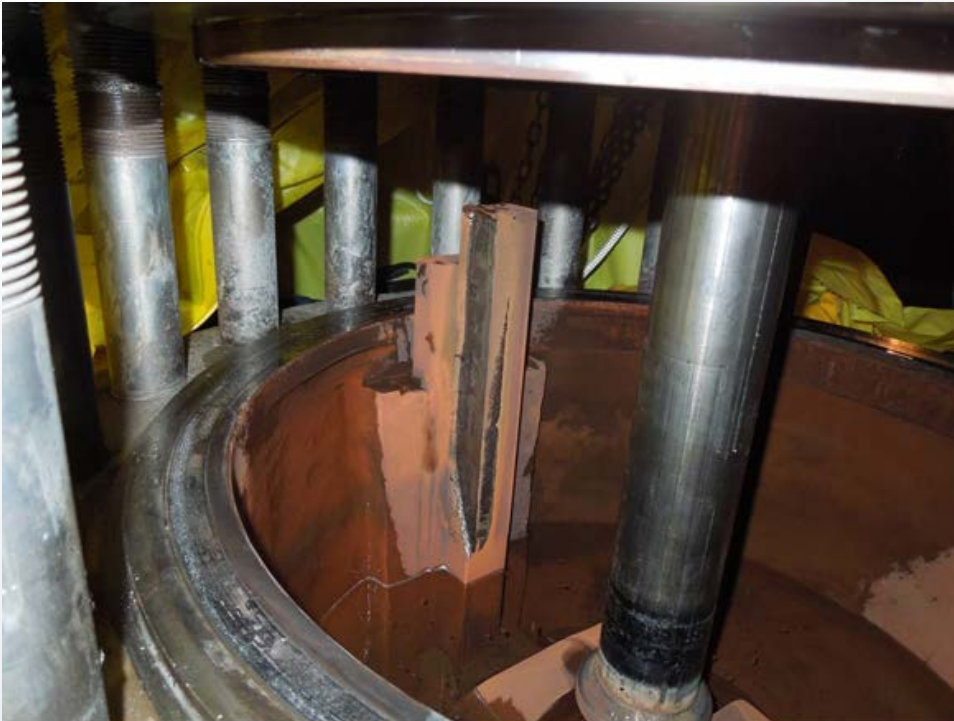
2B33-F067B – Stellite Guide damage (L2R14)
