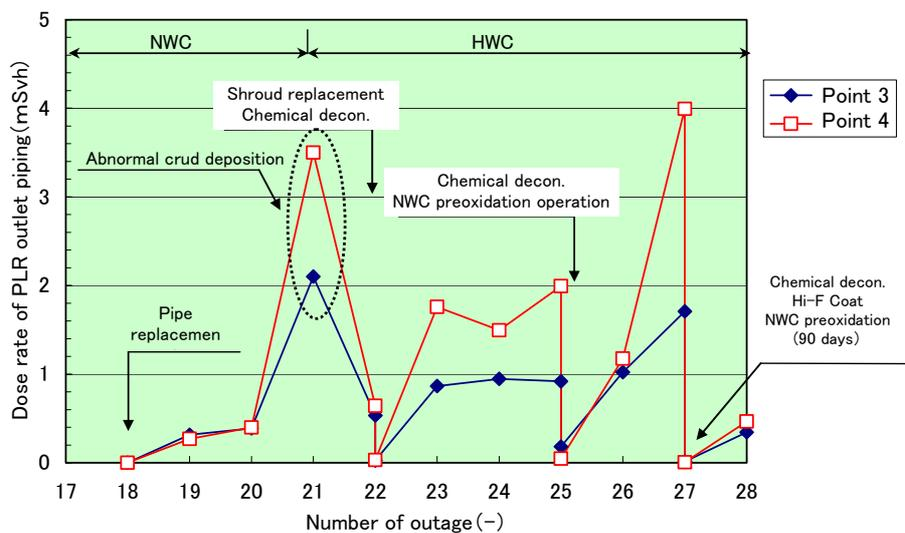
Fig. 4 Dose rate of PLR outlet piping
