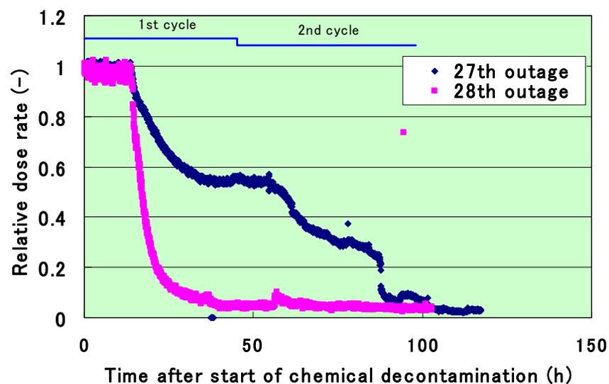
Fig. 5 Effect of Hi-F Coat on chemical decontamination
