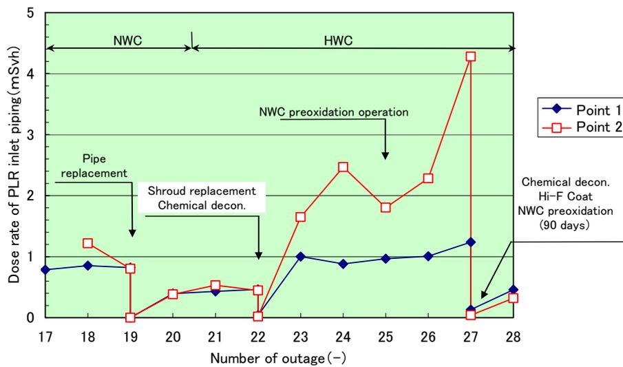
Fig. 3 Dose rate of PLR inlet piping
