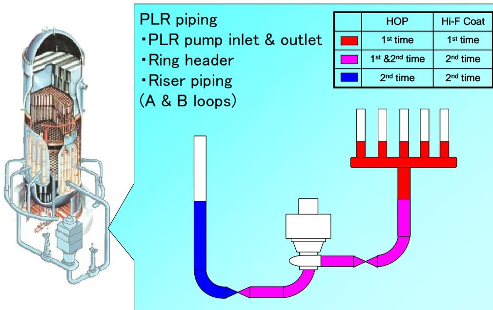
Fig. 1 Application target of HOP decontamination and Hi-F Coat
