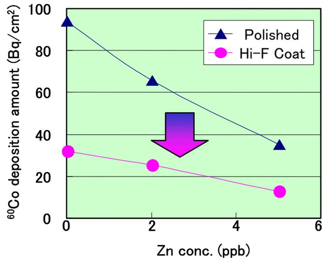
Fig. 6 Co deposition reduction of Hi-F Coat with Zn injection
