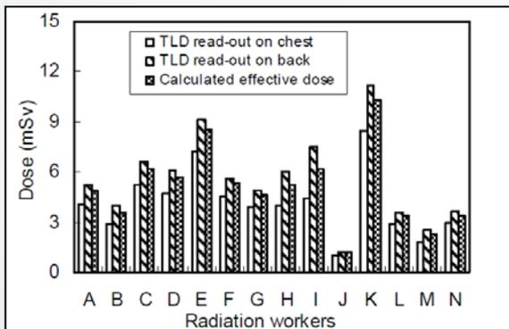
**Fig. 4.** TLD readouts for the installation of a steam generator nozzle dam at Yonggwang NPP No. 1.
