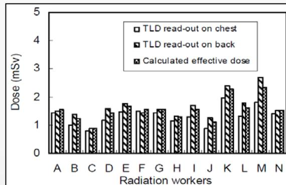
**Fig. 5.** TLD readouts for the plugging and nozzle dam removal of steam generator at Yonggwang NPP No. 1.
