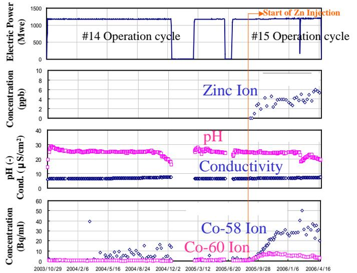
Fig.2 Primary Water Chemistry during the Zn Injection
