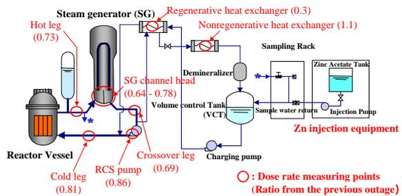
Fig.3 Relative dose equivalent rate on the primary equipment and pipes
