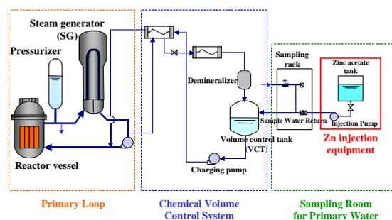
Fig.1 Zinc Injection System in Tsuruga-2
