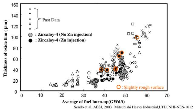
Fig.4 Measured thickness of oxide film
