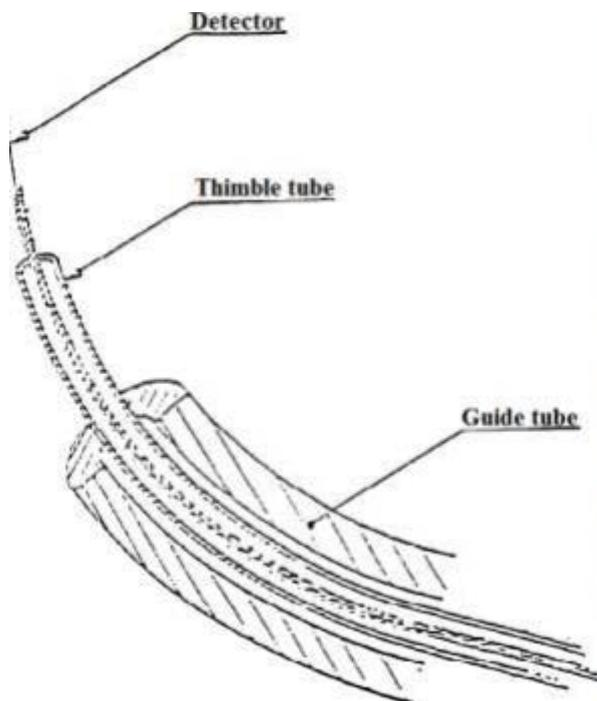
Figure 2: Guide tube pattern
