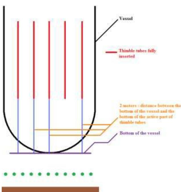
Figure 5: Thimble tubes fully inserted
