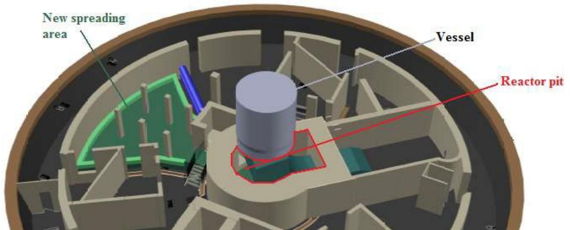
Figure 8: Overview of reactor pit and new spreading area
