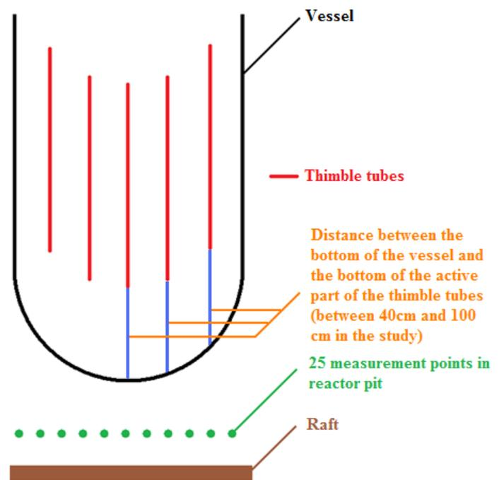
Figure 6: Thimble tubes partially inserted
