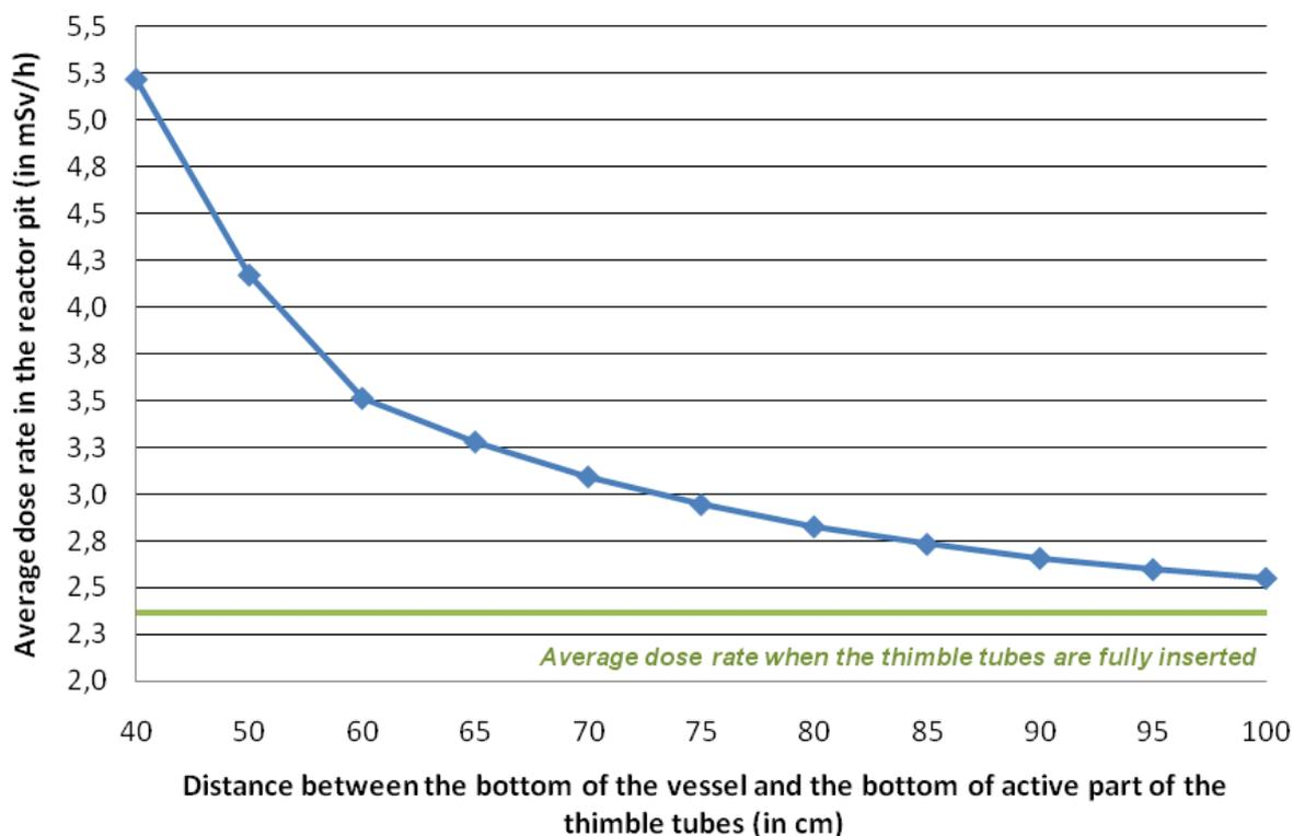
**Figure 7: Average dose rate in the reactor pit as a function of position of the thimble tubes**
