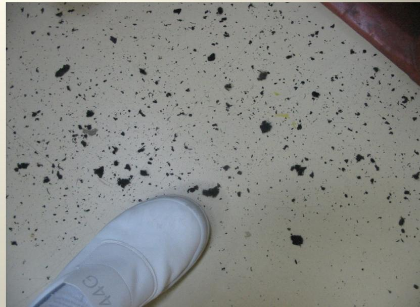
Incandescent particles (insulation material) were projected from the outlet. • The material temperature (post filter and iodine trap) increased by convection through the metal casing (separating the heating system of discharging casing). The temperature was high enough to carbonize and reach the point of ignition.
