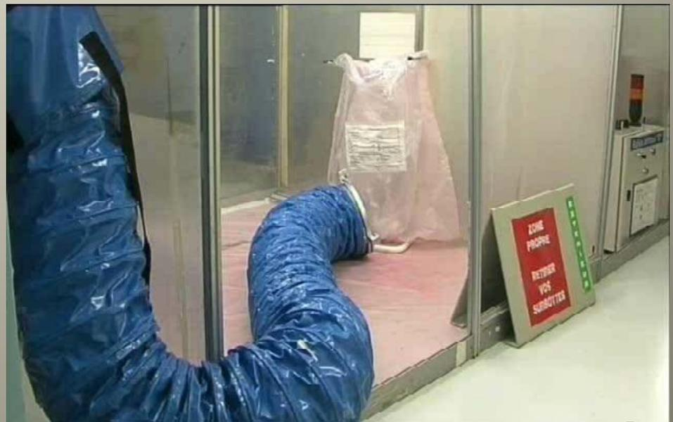
**Fire:** Some specific Portable Ventilation Units are equipped with High Efficiency Filter (aerosols) + Iodine Trap. Obstruction of the suction duct can also be the cause of overheating and thus fire can almost start. Heating system is used to increase temperature and ensure relative humidity lower than 40%, upstream iodine trap (OE Tricastin).
