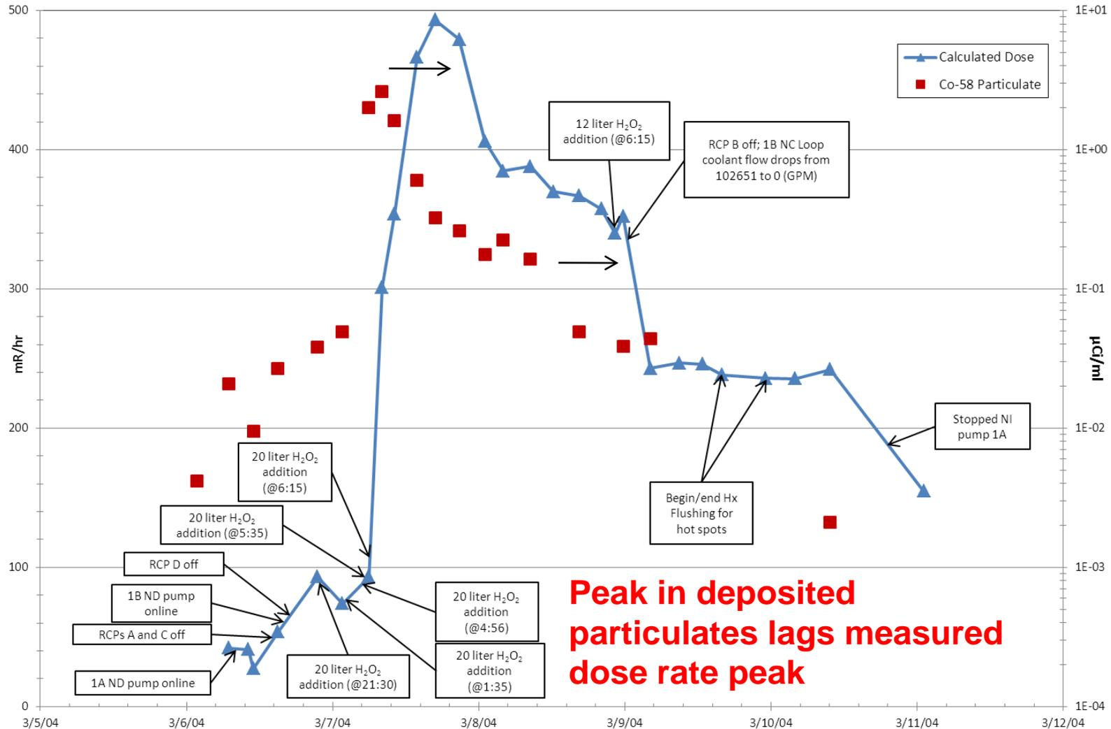
**Peak in deposited particulates lags measured dose rate peak**
