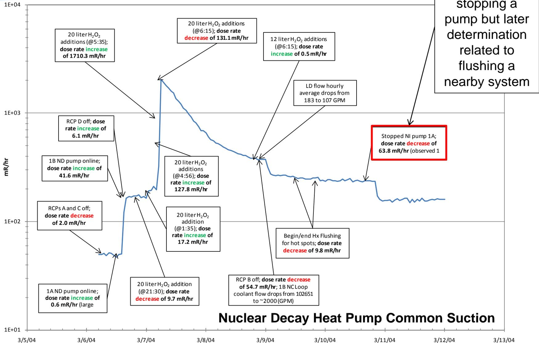
Drop originally attributed to stopping a pump but later determination related to flushing a nearby system
