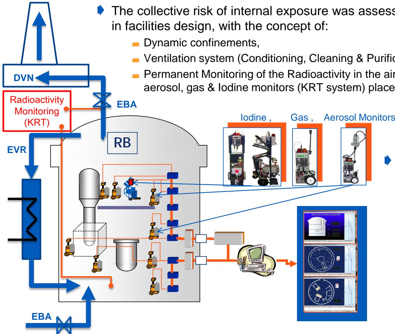
▶ In complement, EDF has set up a network of fixed and mobile Continuous Air Monitors (CAMs) which is giving a near-real-time monitoring of atmospheric contamination in RB.
