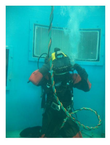
Diver testing comfort of iMUX and electronic dosimetry
