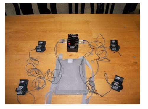
DMC-2000 electronic dosimeters connect to the iMUX Transmitter
