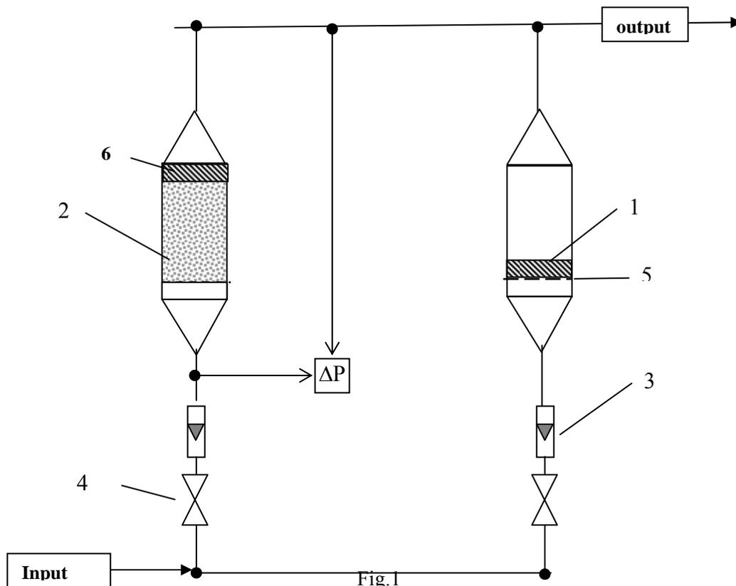
In the figure 1 we have designated as position 1 and 6 – Petrianov filter; as a position 2- BGF; as a position 3 – rotameter; as a position 4 – valve; as a position 5 – the grid; as a  $\Delta P$  - liquid differential manometer;
