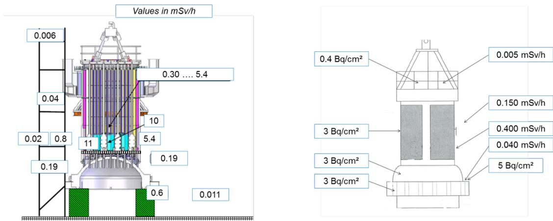
**Figure 1 – Dose rate and contamination measurements of the RVCH of Tihange 3 (left) and Doel 4 (right).**
