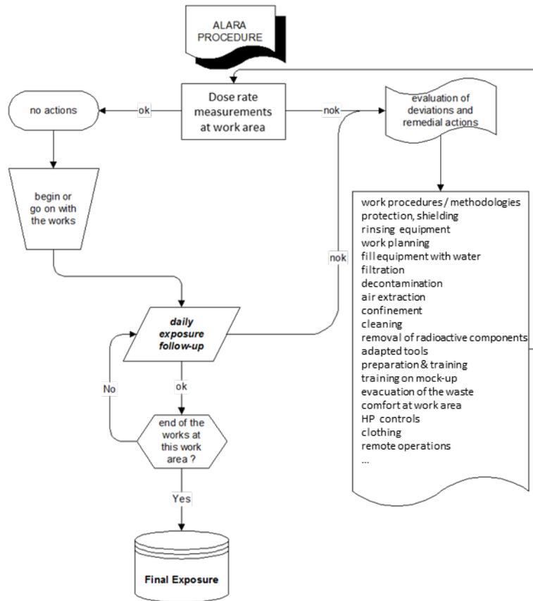
**Figure 3 - Flow chart of the ALARA procedure implemented for the replacement projects.**
