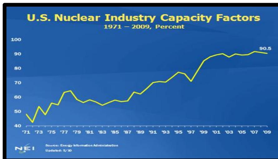
U.S. Nuclear capacity factor, a measure of efficiency, outpaces all other forms of electric generation in the U.S. Coal, for instance, which is the leading source of U.S. electric generation, had a capacity factor of 63.1 percent last year, natural gas 43%, hydro 29%, wind 28%, and solar 24%. [2]
