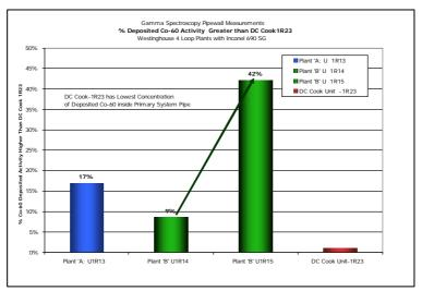
Finally, the gamma spectroscopy pipe wall measurements on Unit 1 this spring, shown above, provided quantitative evidence of Cook's low Co-60 deposition on primary piping compare to other 4 Loop Westinghouse PWRs with Inconel 690 Steam Generators:
