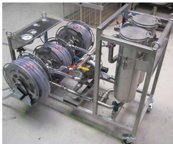
Figure2: Cleaning skid with rolled reinforced tubes prepared for transportation
