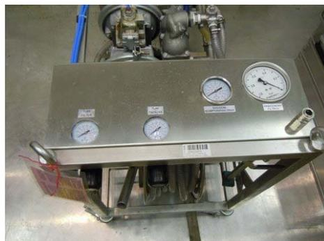
Figure 4: Control panel with pressure indicators
