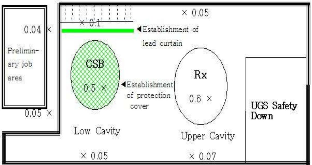
[Picture 9)] Radiation dose rate of Rx cavity area
