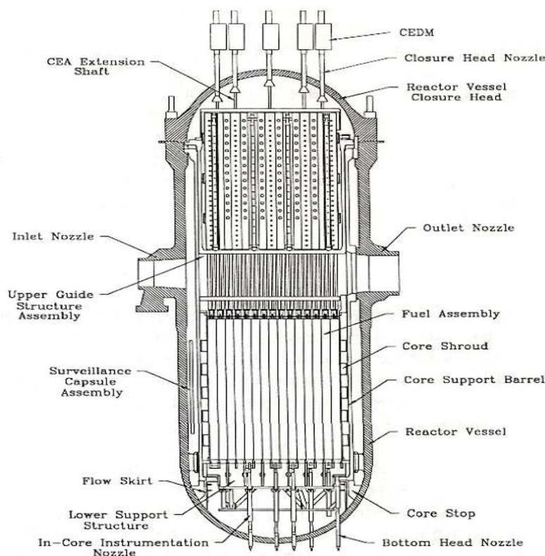
[Picture 1] The Design of Rx Vessel
