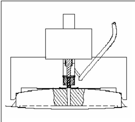
[Picture 18] The execution of leak test
