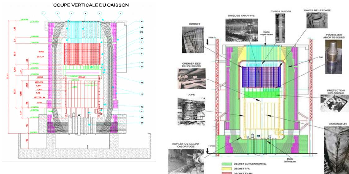
Dismantling scenario and principles for Bugey 1 - Underwater dismantling of internal equipment
