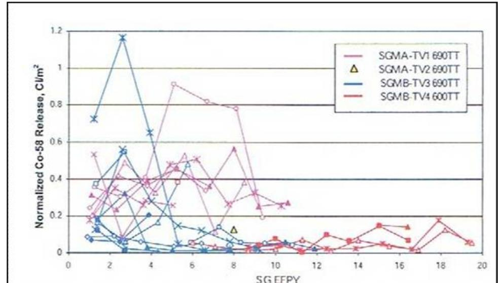
The application of a rigid Cobalt Reduction Program to minimize the cobalt entry into the plant and review of SG tubing or other replacement materials is essential in the long term aspects of operation and impact on source term
