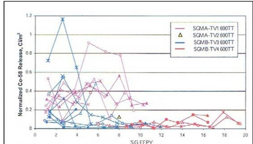
Shutdown chemistry not performed consistently and with proper controls can and as resulted in significant particulate releases. These releases will create significant issues related to outage dose
