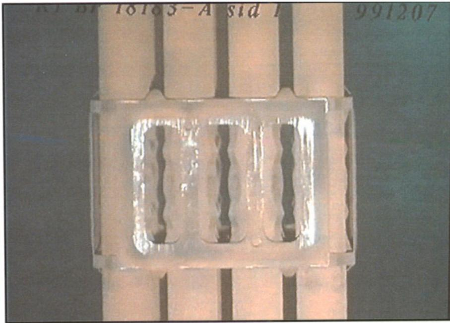
Spacer six before decontamination
