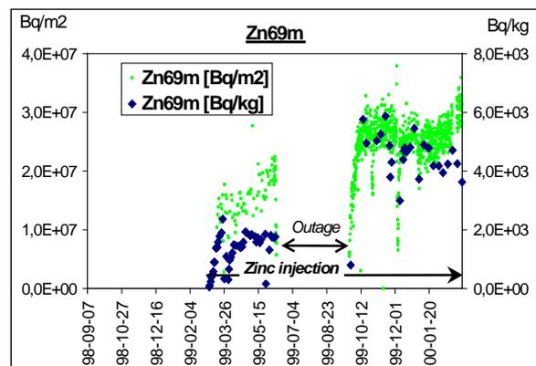
Figure 8 Zn69m in B2. OLA and reactor water.
