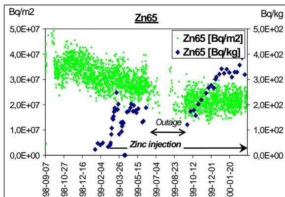
Figure 7 Zn65 in B2. OLA and reactor water.
