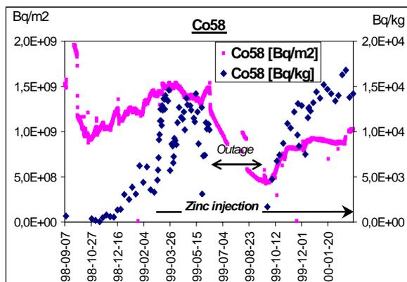
Figure 5 Co58 in B2. OLA and reactor water.
