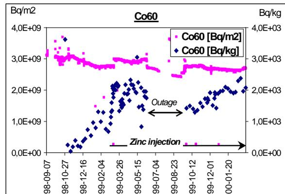
Figure 6 Co60 in B2. OLA and reactor water.
