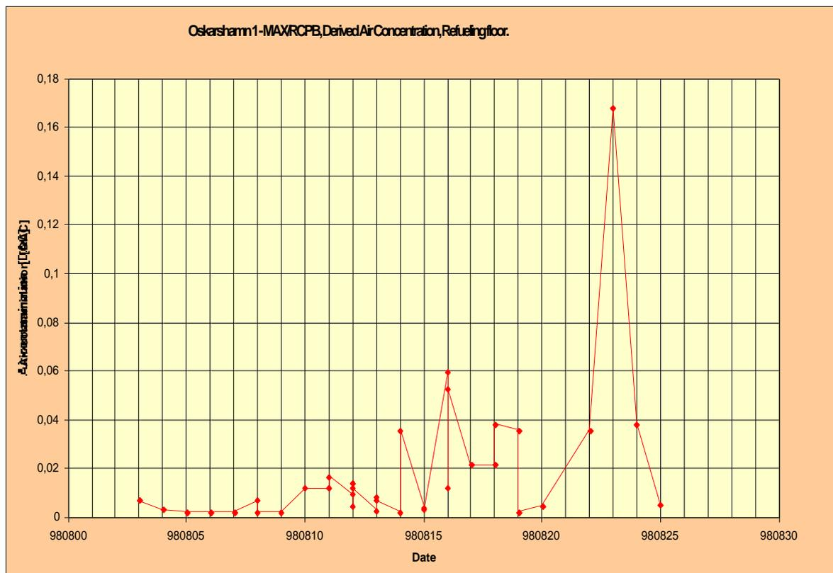
Figure 5, measured air contamination on refuelling floor.
