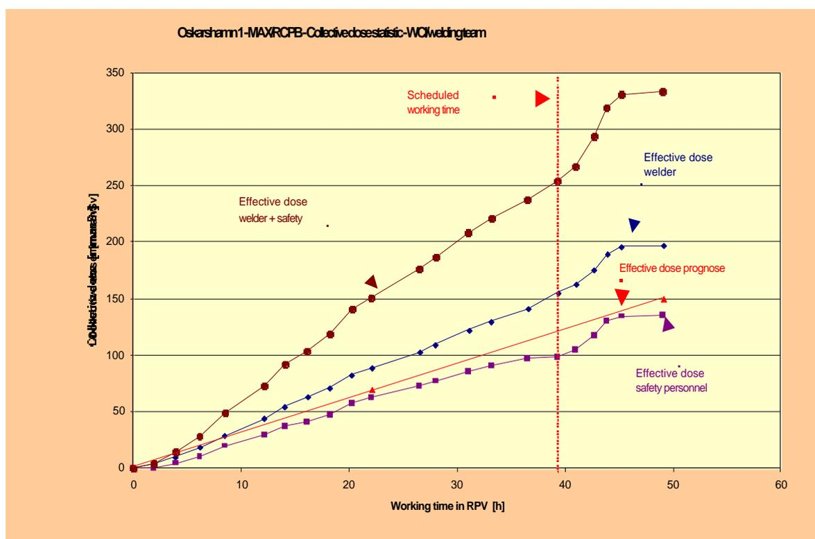
Figure 3, Effective dose statistics for the welding task.
