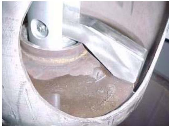
Control Rod Guide Tube (CRGT) Flush Tool at Dresden
