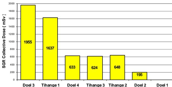
The dose allocated to this replacement of the steam generator was kept to 195.5 man-mSv. This success was the result of experience from previous replacements, a successful decontamination of the primary circuit, a well studied shielding with 70 tonnes of lead, and operational planning with a maximum attention to ALARA, for example: keeping the steam generators, that had to be replaced, filled with water for as long as possible.
