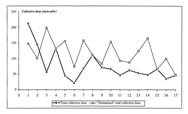
Figure 1 Evolution of the collective dose for the machining of RHR exchangers
