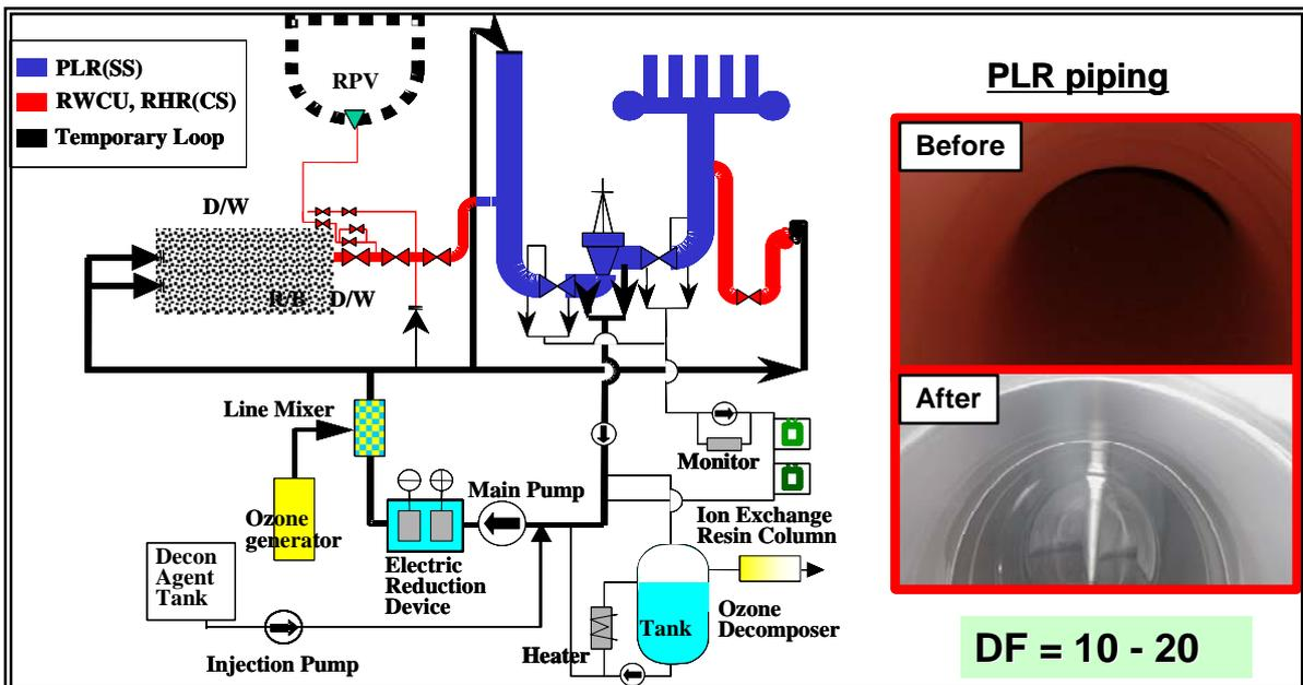
Fig. 3 Application of T-OZON to system decontamination in a BWR
