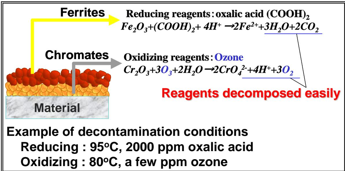
Fig. 2 Principle of T-OZON
