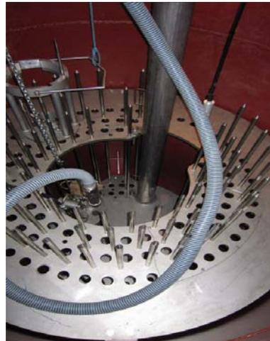
Mock-up of upper support plate with heaters
