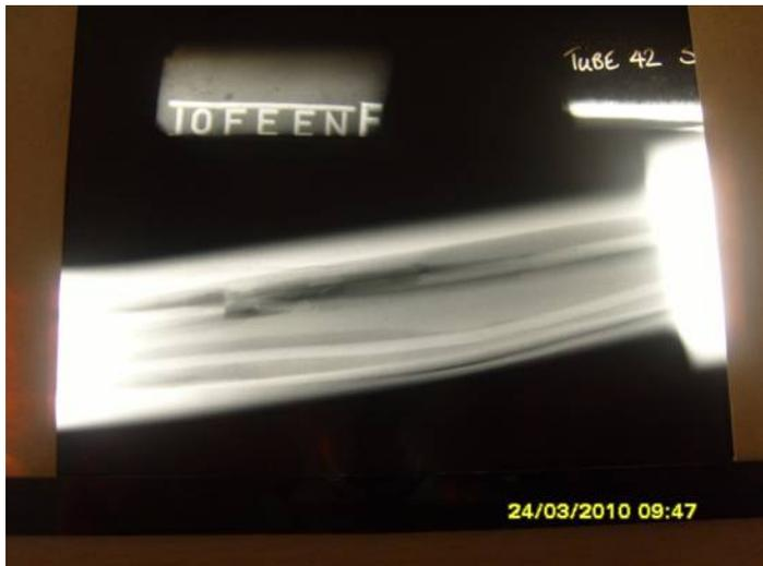
Heater 42 Radiograph showing disruption to the heater and the HWI
