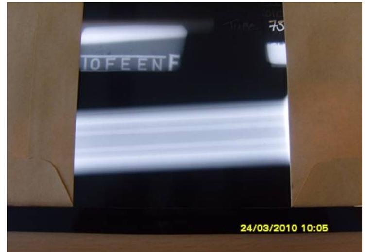
Heater 72 Radiograph showing a normal heater and HWI
