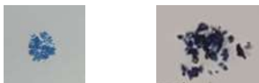
Figure 1. 6-BU sample before (left) and after (right) alpha irradiation
