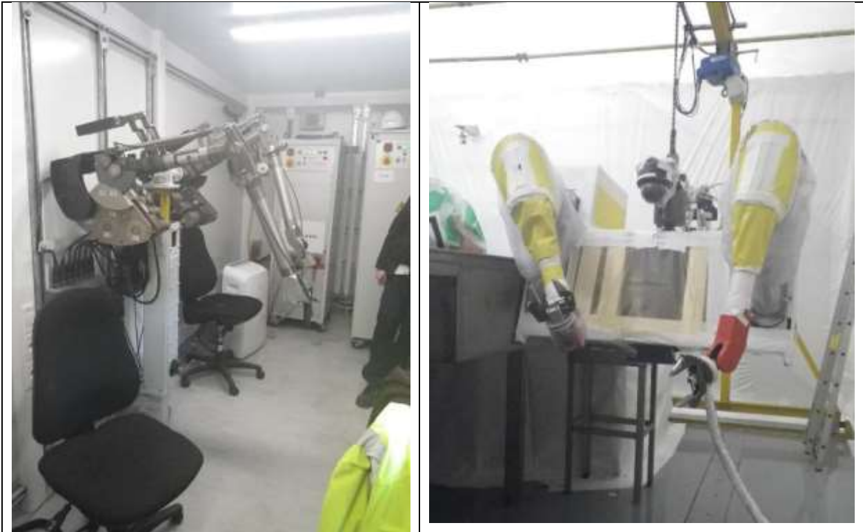
Figure 2: Left: master slave arms used by the operator inside the shelter (outside of the RCA). Right: pictures of the robot ready for use in its confinement
