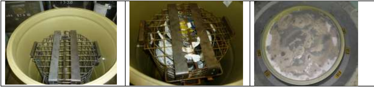
Figure 4: from left to right, view of a final waste drum at 3 main stages: (i) empty final waste drum, (ii) fulfilled final waste drum, (iii) conditioned final waste drum with a certified mortar
