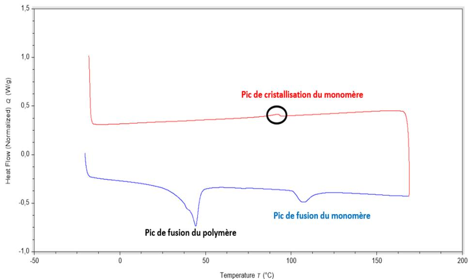
**DSC** : thermal analysis technique. It measures the difference of heat exchange between the sample and a reference => enthalpy. The area of the monomer melting peak is linked to the amount of monomer present in the sample.
