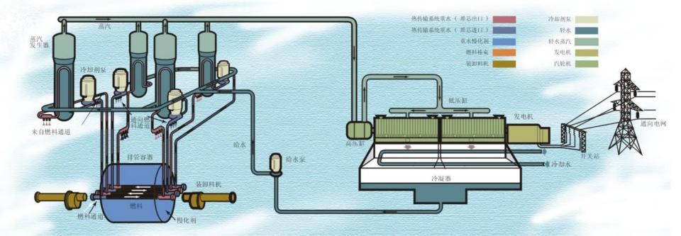
Coolant: ~200T heavy water; Moderator: ~260T heavy water
