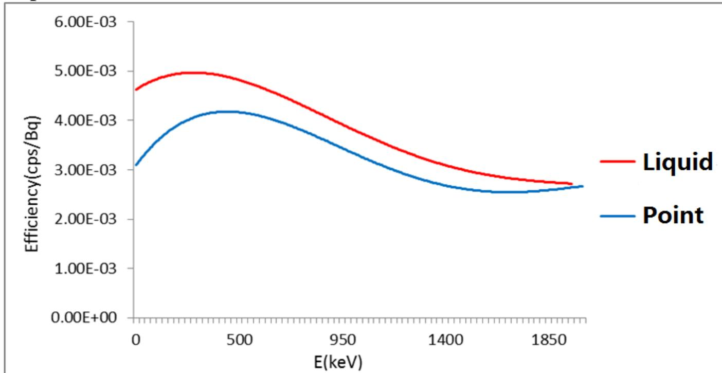
Use MCNP4 simulate liquid source calibration experiment :
