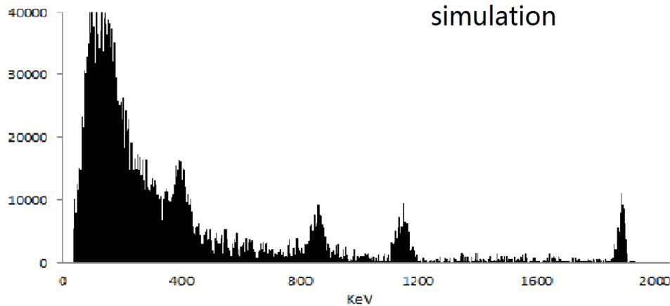
1. The actual Gaussian broadening parameter selects  $^{113}\text{Sn}$ ,  $^{54}\text{Mn}$ , and  $^{65}\text{Zn}$  in the middle;
