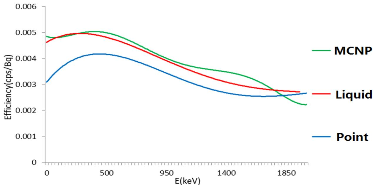
We do two calibration experiments: the liquid source calibration and the point source calibration. And the efficiency result is basically the same. We build liquid source calibration model of MCNP simulation.
