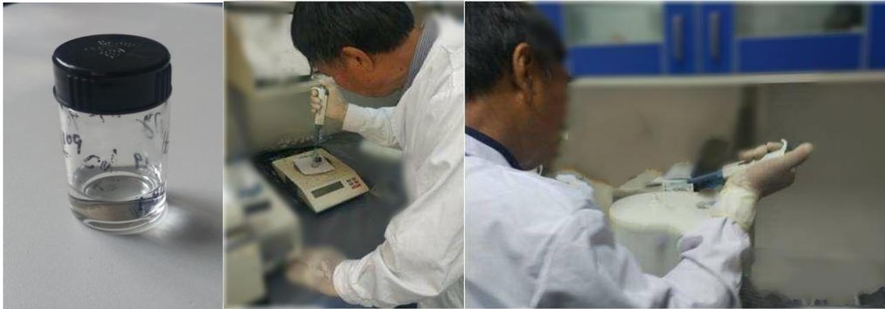
The liquid sources are filled according to the  $\gamma$  ray energy of the liquid source from low to high, and each filling of sources is used for a set of measurements. And then fill next source.
