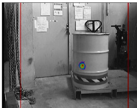
**Fig. 5: Example of localization of a radioactive hot spot inside a 220 l nuclear waste package. The measurement duration is equal to 1 s. The dose rate near the hot spot is about  $300\text{ }\mu\text{Sv}\cdot\text{h}^{-1}$ .**
