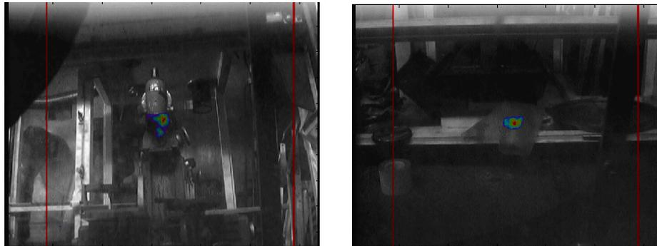
**Fig. 6: On the left: identification of a radioactive hot spot on the top of a milling machine. On the right: identification of a radioactive hot spot contained in a bag.**
