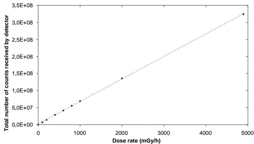
**Fig. 4: GAMPIX's counting rate according to the dose rate received by the camera. The average counting rate is calculated over 10 s of acquisition time.**
