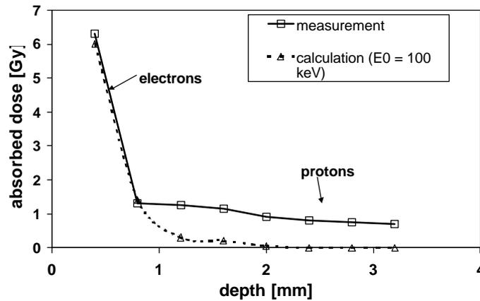
Fig. 1. Gradient of dose measured at the surface of space station MIR (Schöner et al, 1999).
