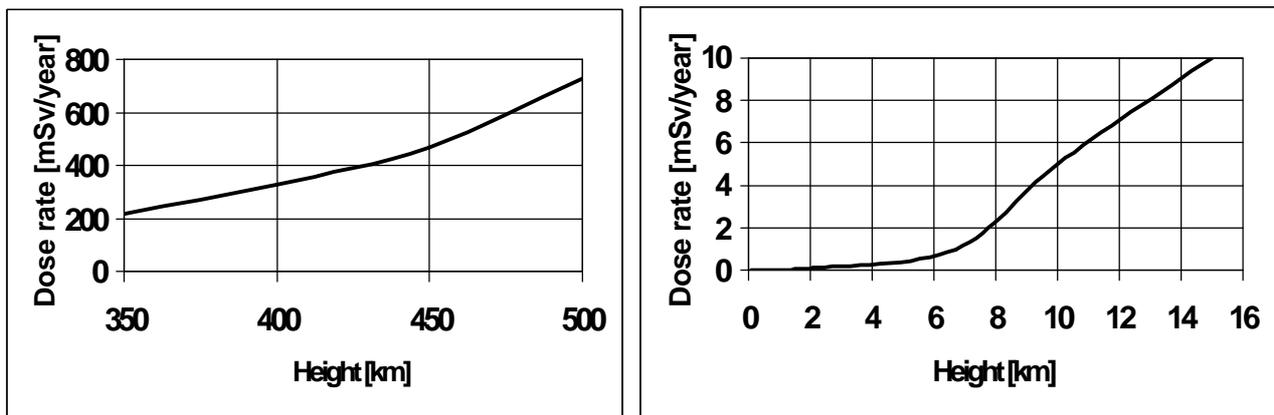
Fig 2. The expected average annual dose as a function of flight altitude for case of orbital stations (a–left) and aeroplanes (b–right).
