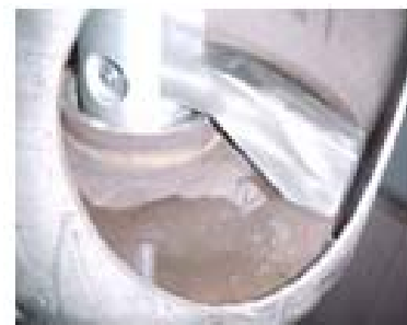
(CRGT flush tool 95% inserted with Nozzle deploying)
