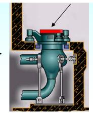
2. The working area of the opened (i.e. without electromotor) pump elbow was characterized by the dose rate near 2,5 mSv/h.
