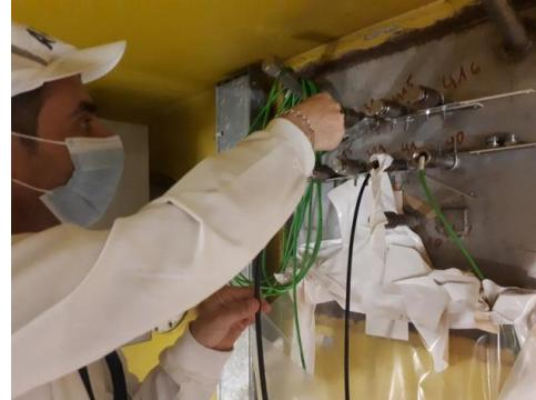
*Insertion of OSL probes inside guide tubes*
