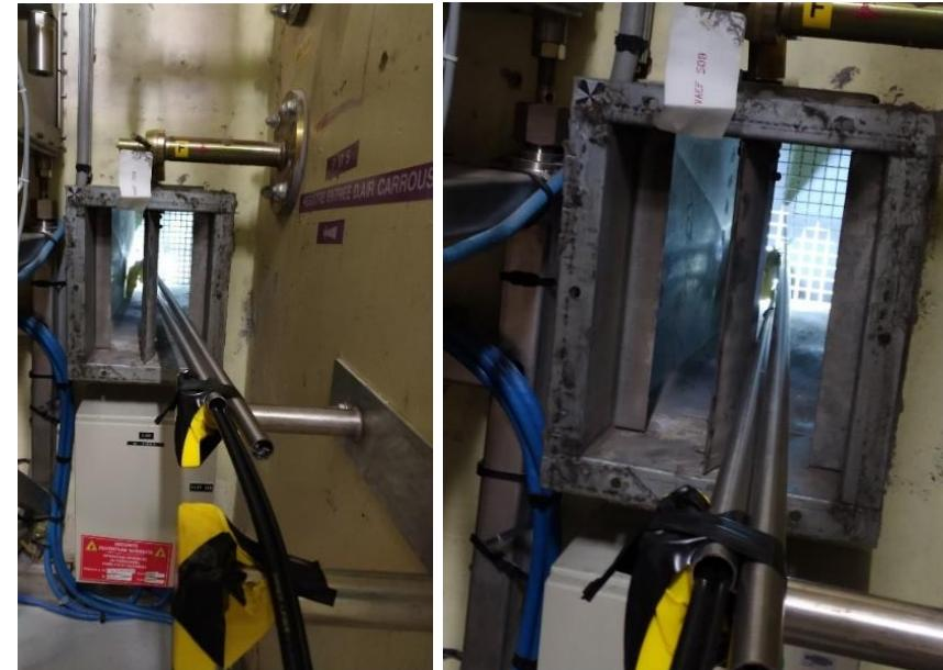
*Insertion of OSL probes through the aeration grid*
