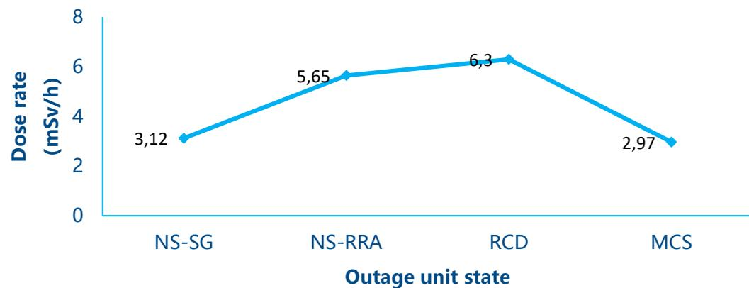
During unit first outage, the contact dose rate of H4PTR404TW before fuel unloading was much lower than that after loading fuel. The Replacing of H4PTR404TW sealing ring was firstly arranged after loading. The work was rearranged to the time before unloading, and about 0.5 man ·mSv was optimized.
