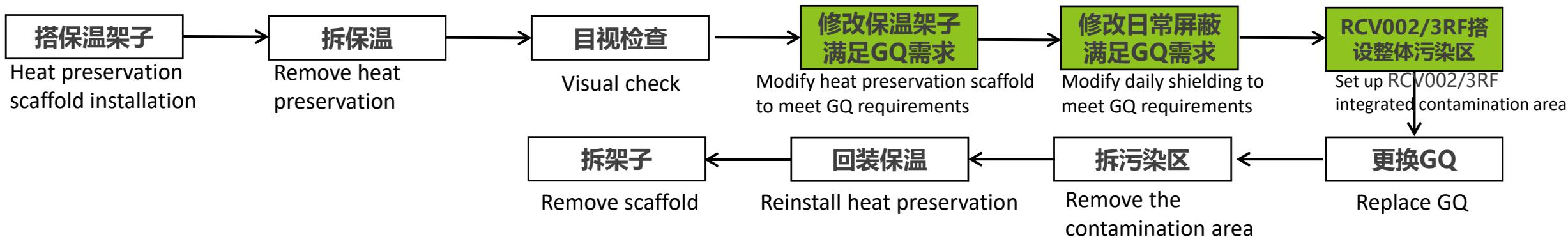
One time of shielding construction and removal + one time of heat preservation removal and installation, 80% of scaffold erection time and 40% of site erection time are reduced by this optimization.
