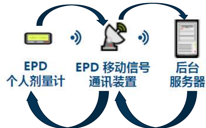
Fig2.the main structure of the system
